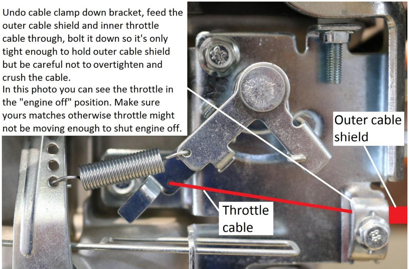
Make sure that when the throttle cable lever is in its "full choke" position that the choke rods circled in red here are being pushed in all the way (or as close to it as possible) to correctly activate the choke.
